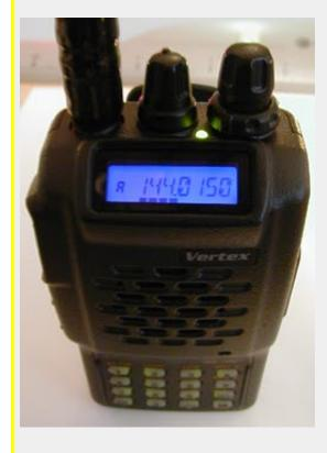
My VX-150 with the LCD display LED changed to Blue. The original LED was removed and replaced with a blue SMT LED (1206 size). R1239 (2200hm) was removed and replaced with a 0 0hm resistor.
