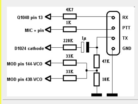
Due to existing varicap diode modulator we'll need only very few new parts. The correct values are found after modifying 4 set of FT-50 radios. Because of space restriction I suggest the use of a (47k/10k) resistive voltage divider and not even the smallest pot. You can increase the value of the 1uF capacitor to improve low-frequency response.
