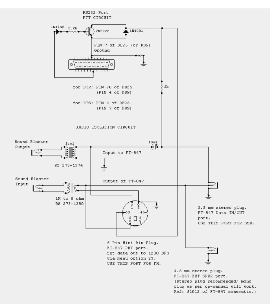
**Note.** Due to the low voltage output levels of the PKT and Data IN/OUT ports, it is recommended to use the EXT SPKR port as output to the sound blaster. This will ensure proper SSTV signal triggering and synchronization.
