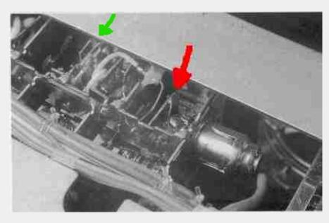
3. On the figure, next to the red arrow, there's a horizontal copper strip, with another vertical copper strip strip soldered at its end. These two strips make an angle of  $90^{\circ}$ .
