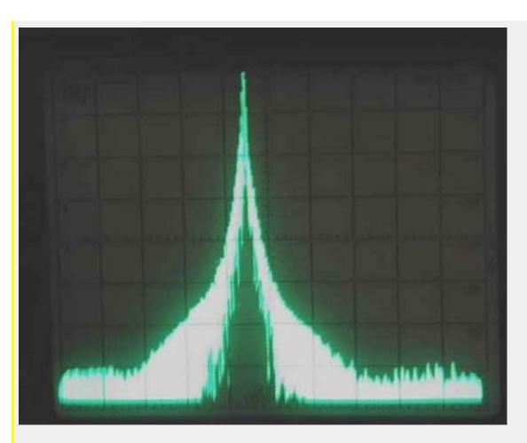
The 751A is approximately -58 dB at 1 kHz, and rolls off smoothly. Here is the nicely sloped (but too fast) 751A rise:
