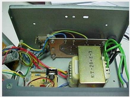
Photo 5: Position of speed reduction PCB
