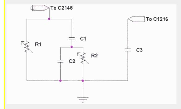
C3 was a .1uF disk capacitor. This component's value turned out to not be especially critical, it mainly prevents fast rise and fall of the low-level RF amplifier stage that is driven by a gate. There was no combination of resistance across or in series with this capacitor that reduced clicks in any of the radios I tested.
