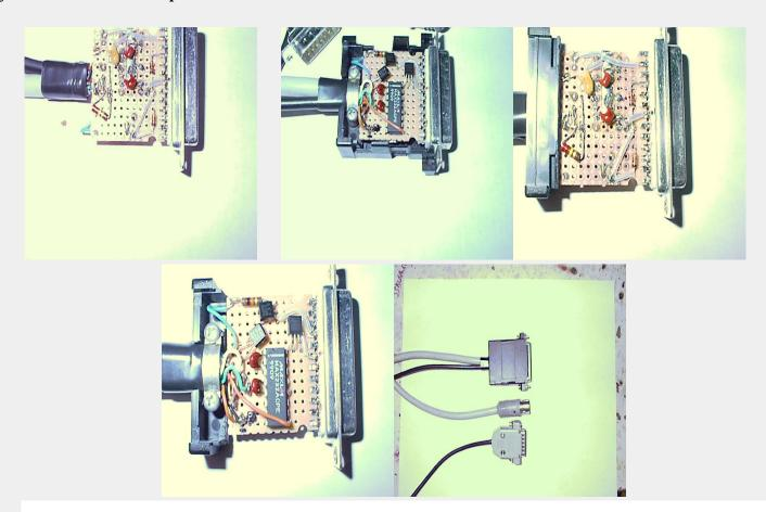
FRG-9600 self powered, self contained, (in a DB25 snap together shell) RS232 to TTL/CMOS voltage level translator.
