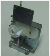
Photo 3: Mechanical indicator needle system
