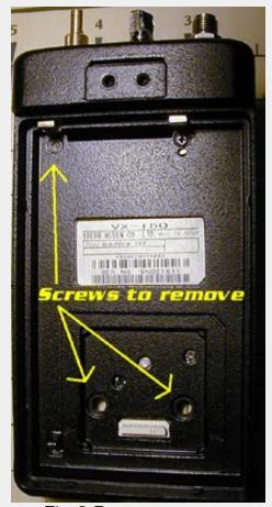
Fig 2 Remove screws
