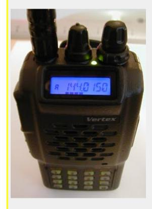
My VX-150 with the LCD display LED changed to Blue. The original LED was removed and replaced with a blue SMT LED (1206 size). R1239 (2200hm) was removed and replaced with a 0 0hm resistor.
